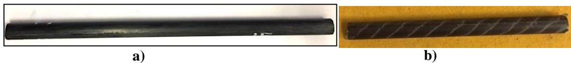
Figure 59 a) Unidirectional rod sample "UD", b) 3D helical twisted rod sample "Corda"
