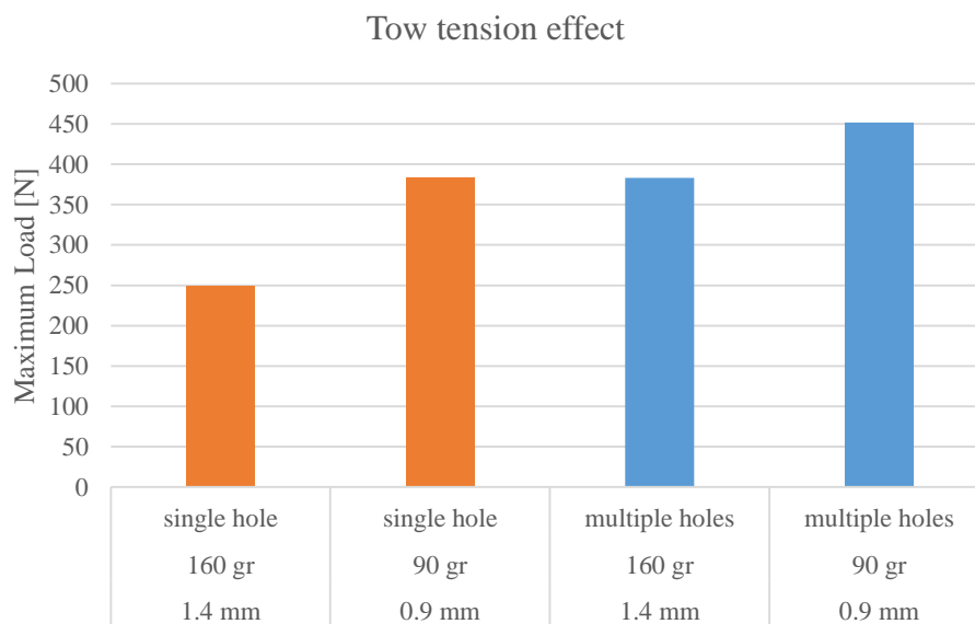
Figure 46 - effect of the tension on each tow for both the single and multiple holes configurations
