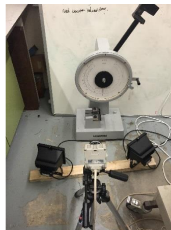
Figure 68- Charpy test: experimental apparatus and test setup
