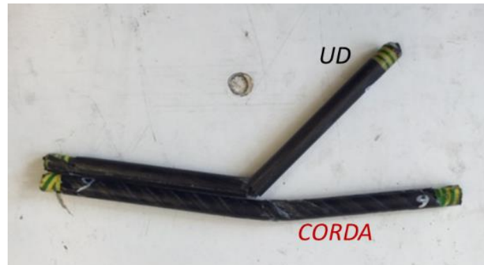
Figure 67 - post impact behaviour of unidirectional and twisted samples
