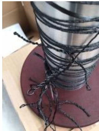
Figure 47 Single strand (200 tpm first twist) showing corkscrew defect
