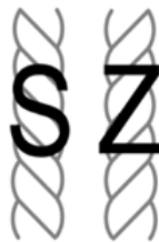
Figure 39 Illustration of the S and Z naming convention [197]
