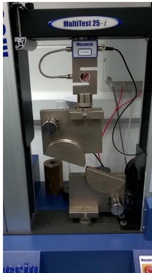
Figure 50 Tensile machine for testing cordages (Bridon International Technical Centre)
