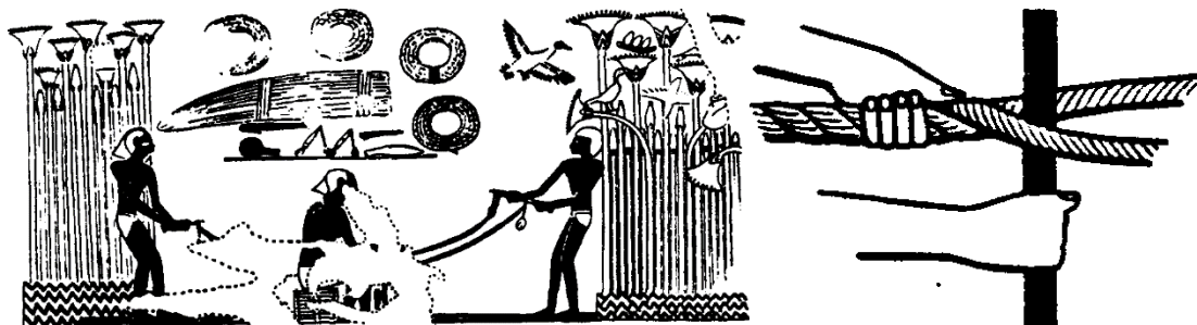
Figure 26 Figure 285—(Left) Rope-laying. From a tomb at Thebes, c 1500 b.c. (Right) Detail showing how the man in the centre controls the closing of the two strands, reproduced from [182]
