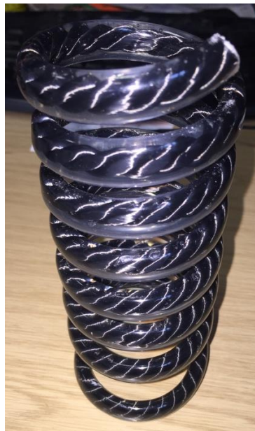
Figure 155 Helical-Spring made using the 3D helical twisted fibre reinforcement
