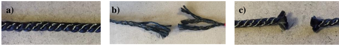
Figure 32 a) three strands cordage with Nitinol wires inserted in the first stage; b) fraying of the strands after cut the cordage without activating the Nitinol wires; c) unravelling effect of the cordages after activating the Nitinol wires
