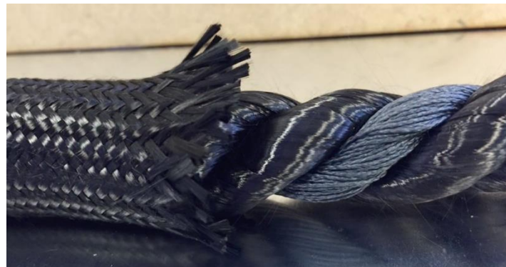
Figure 56 Three strands rope with external carbon fibre jacket
