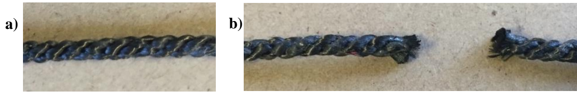
Figure 36 a) three strands cordage with tows treated with adhesive spray; b) unravelling effect of the cordages after cut
