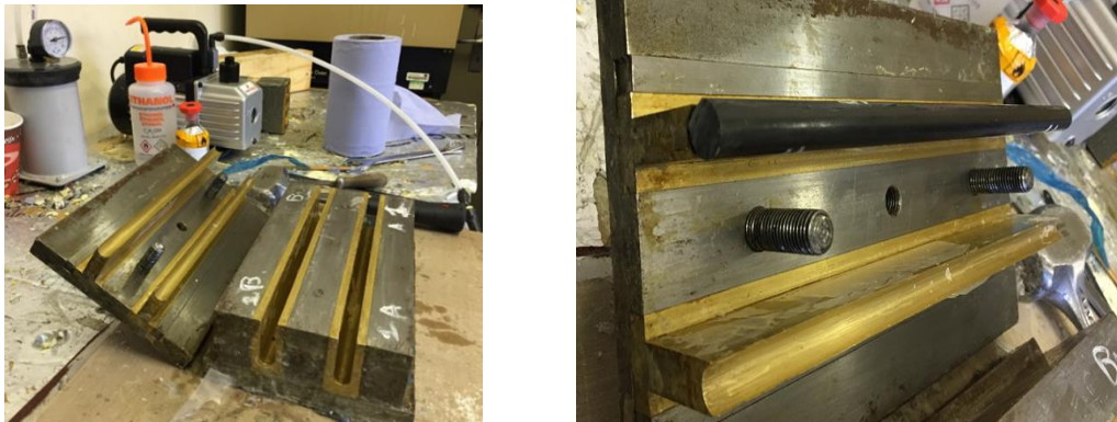
Figure 58 - mould used for the manufacturing of the rods
