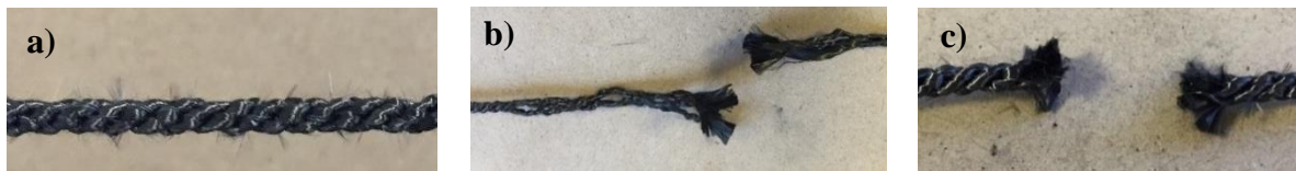
Figure 33 a) three strands cordage with Nitinol wires inserted in the second stage; b) fraying of the strands after cut the cordage without activating the Nitinol wires; c) unravelling effect of the cordages after activating the Nitinol wires
