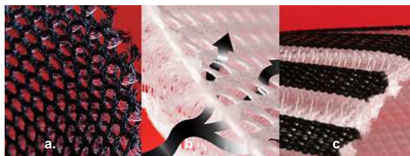
Figure 7: Cross sections of Spacetech textiles by Heathcoat, a and c are two design variations and b illustrates the air flow through the textile.
