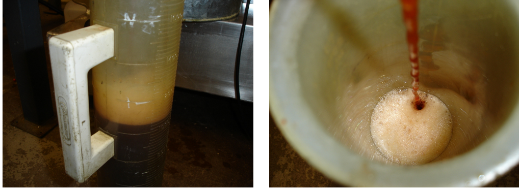
Figure D-18: Frothing issue found during hydrostatic tests
