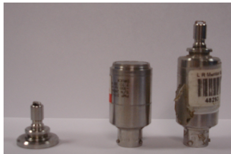
Figure D-11: The machined pressure transducers
