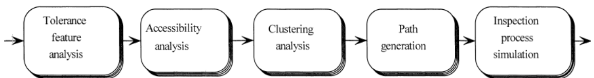
Figure 3-20: Five modules in offline measurement planning (Zhang et al. 2000)
