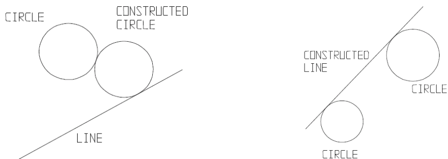
Figure 6-36: Examples of constructed features with tangency relations (ISO 2010c)
