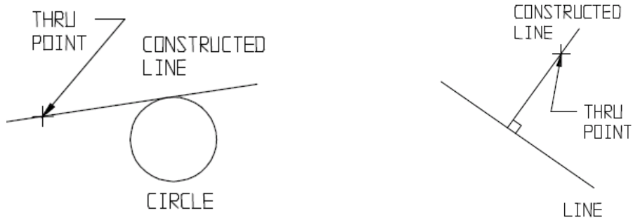
Figure 6-37: Pass through construction examples (ISO 2010c)
