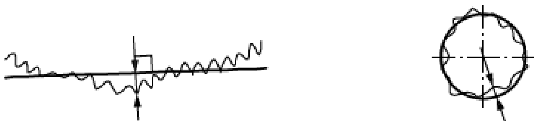
Figure 4-18: Distance based measurement evaluation (ISO 2011j)
