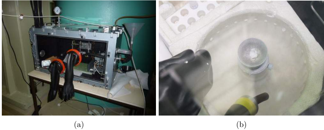
Figure 4-3: (a) The nitrogen filled glove-box used for loading samples at the ILL and (b) top down view of loading ice-Ih into the vanadium can via an aluminium funnel.
