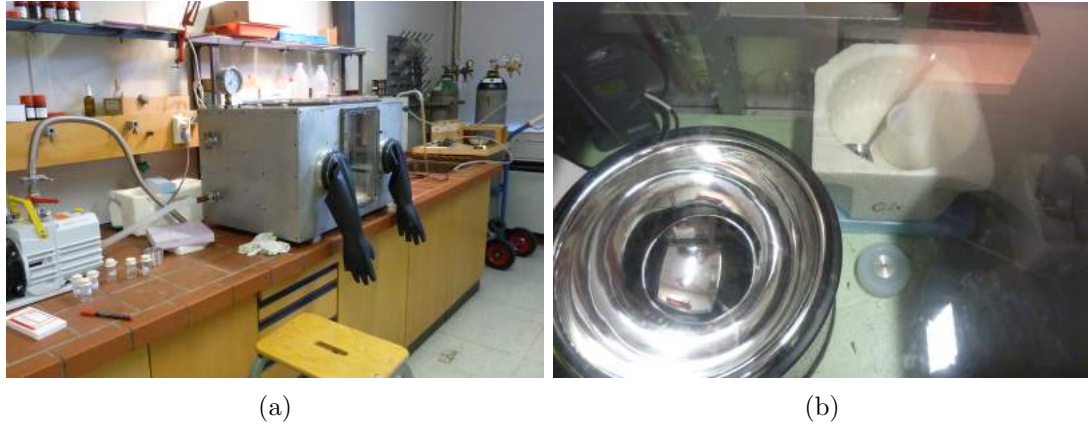
Figure 4-2: (a) The nitrogen filled glove-box used for preparing the ice samples at the University of Göttingen and (b) top down view of the inside of the glove-box showing the sample preparation equipment.
