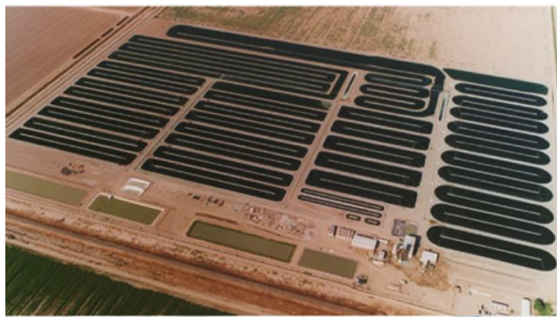
Figure 1.3: Raceway ponds driven by paddle wheels at the Earthrise Spirulina, California, USA. The production plant has 37 Spirulina ponds, each covers 5000 m 2 , and is mixed by 15.24 m paddlewheels in each pond (Earthrise, 2017). The photo is adapted from (Borowitzka and Moheimani, 2013, pp. 133-152).
