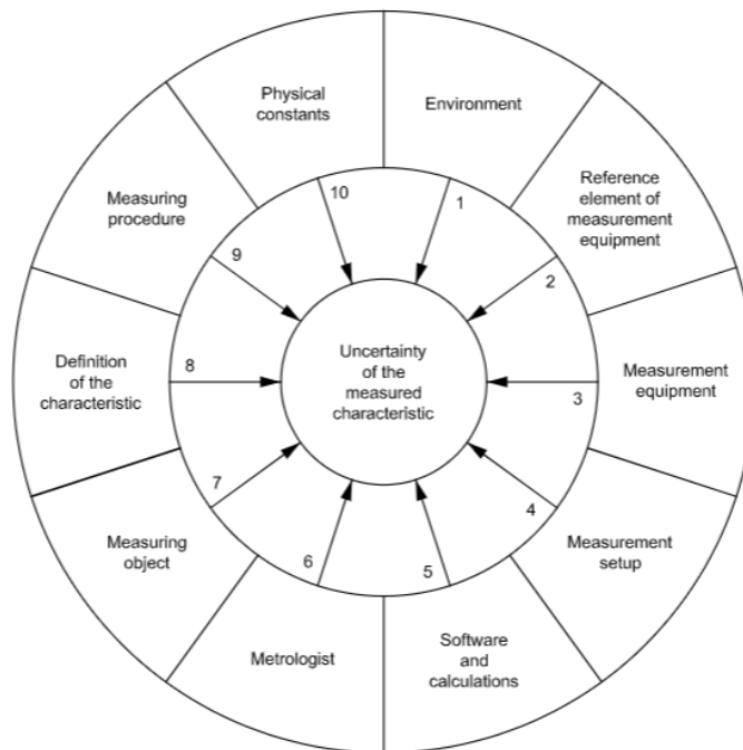
Figure 4 - Uncertainty components in measurement (ISO 14253-2:2011, 2011).
