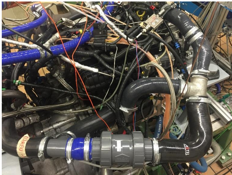
Figure 5.8. Check valve configuration.
