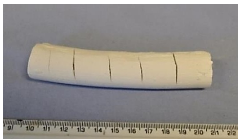
Figure 3.8 Photograph of a 5A zeolite monolith (Sample no. 17) showing the formation of cracks during drying.
