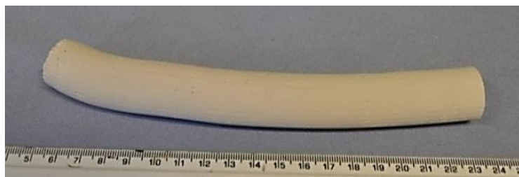
Figure 3.9 Photograph of a bent 5A zeolite monolith (Sample no. 18) during drying.
