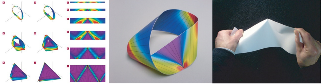
Figure 31 A mathematical treatment to find the shape of a Developable Mobius strip. Images from (Starostin & van der Heijden 2007)
