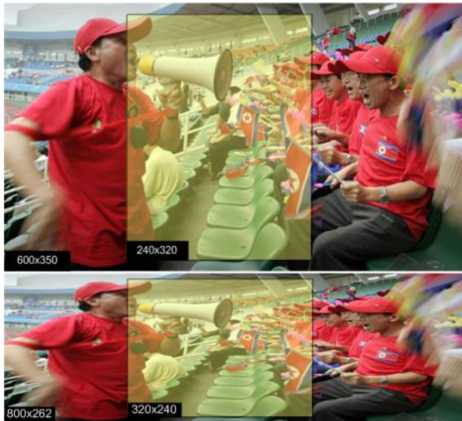
Figure 5.22: The effects of content transformation, as it would appear on a mobile device’s display (yellow area). The top illustration consists of the source image and the lower illustrates the target output.
