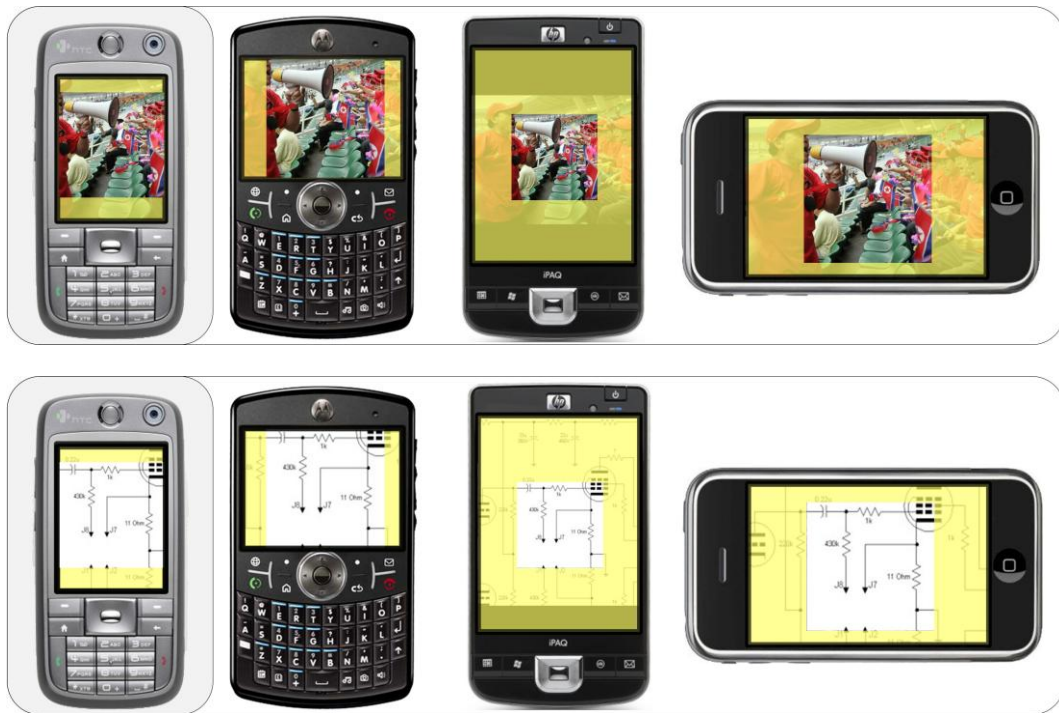
Figure 5.25: Content peripheral framing, across four devices: S730 (source device), Motorola Q9, HP iPAQ 200 and Apples iPhone. Across four common screen resolutions from left to right 240x320, 320x340, 480x640 and 480x320.
