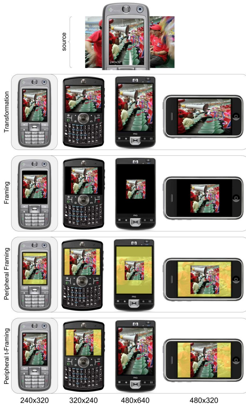
Figure 5.28: An example of image-content transformation (top-row) in comparison to content framing (second-row), peripheral framing (third-row) and peripheral t-framing (bottom-row), across four common screen resolutions 240x320, 320x340, 480x640 and 480x320.
