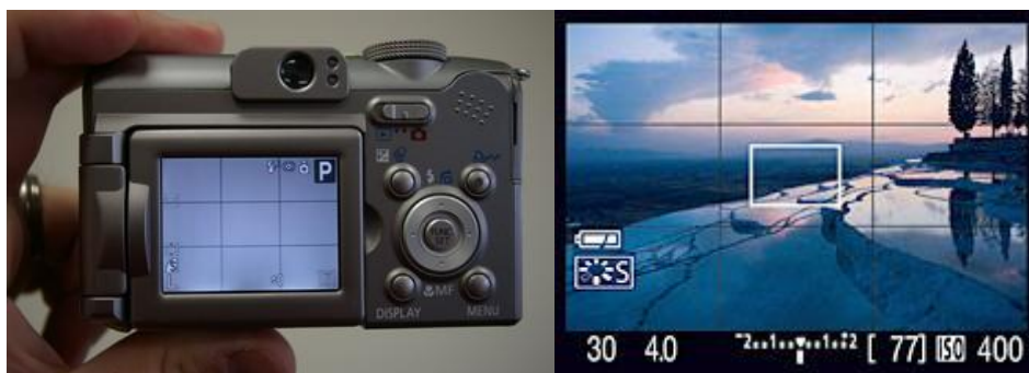
Figure 6.21. Scene framing and alignment grid, a common feature on most digital cameras.
