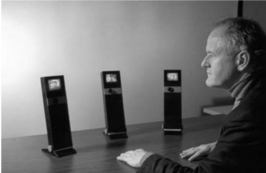
Figure 2.4: The Hydra four-way teleconferencing system.
