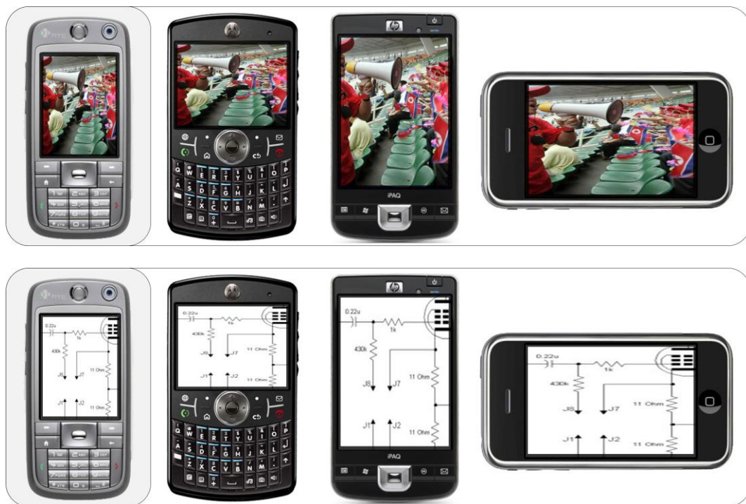
Figure 5.23: Content transformation, across four devices: S730 (source device), Motorola Q9, HP iPAQ 200 and Apples iPhone. Across four common screen resolutions from left to right 240x320, 320x340, 480x640 and 480x320.
