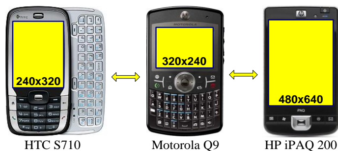
Figure 5.21: Illustrative example of variations in screen resolution and orientation across a number of available Windows Mobile devices.
