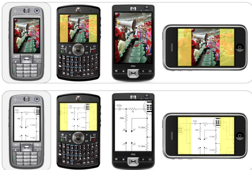
Figure 5.27: Content peripheral t-framing, across four devices: S730 (source device), Motorola Q9, HP iPAQ 200 and Apples iPhone. Across four common screen resolutions from left to right 240x320, 320x340, 480x640 and 480x320.
