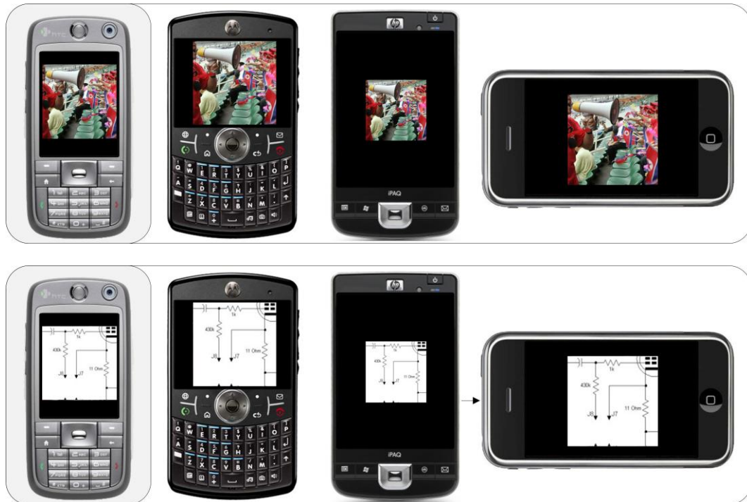
Figure 5.24: Content framing, across four devices: S730 (source device), Motorola Q9, HP iPAQ 200 and Apples iPhone. Across four common screen resolutions from left to right 240x320, 320x340, 480x640 and 480x320.
