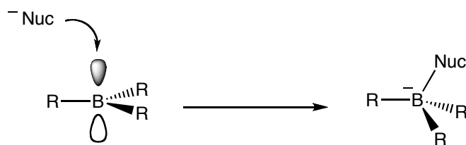
Scheme 5 Diagram showing the change in geometry undergone at the boron centre when the vacant p orbital is filled by an attacking nucleophile.
