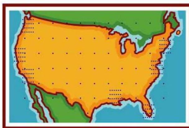
Figure 4.1 – Nominal (low-density) and harbor entrance approach (high-density) ASF grid (Illustration from [52])
