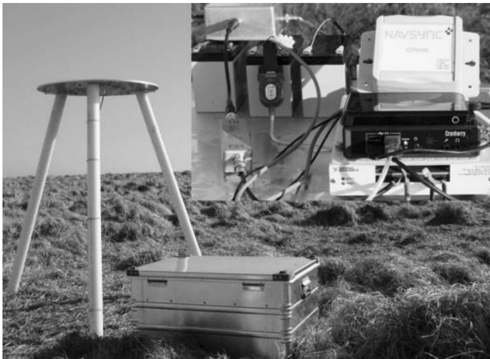
Figure 5.6 – The wide-band digital low-frequency radio receiver used for recording Loran-C signals (Photograph from [59]).
