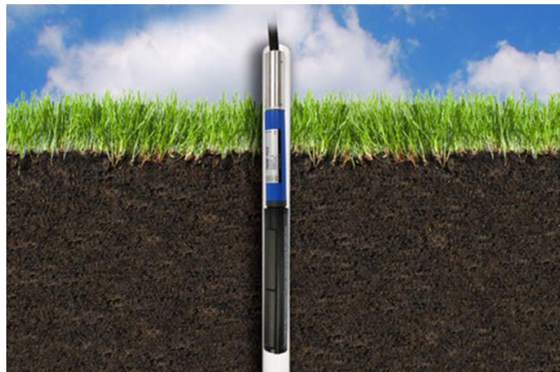
Figure 2.2 – Measuring soil moisture using soil conductivity probe (Image from [25])
