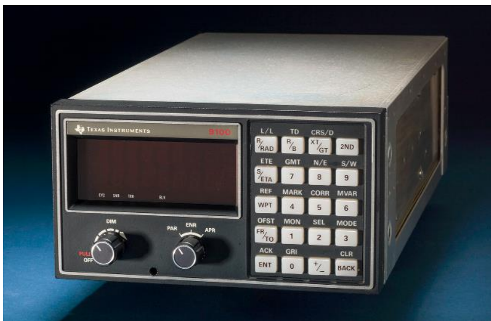
Figure 3.14 – Texas Instruments TI9100 Loran-C receiver (Photograph courtesy of National Air and Space Museum, Smithsonian Institution).
