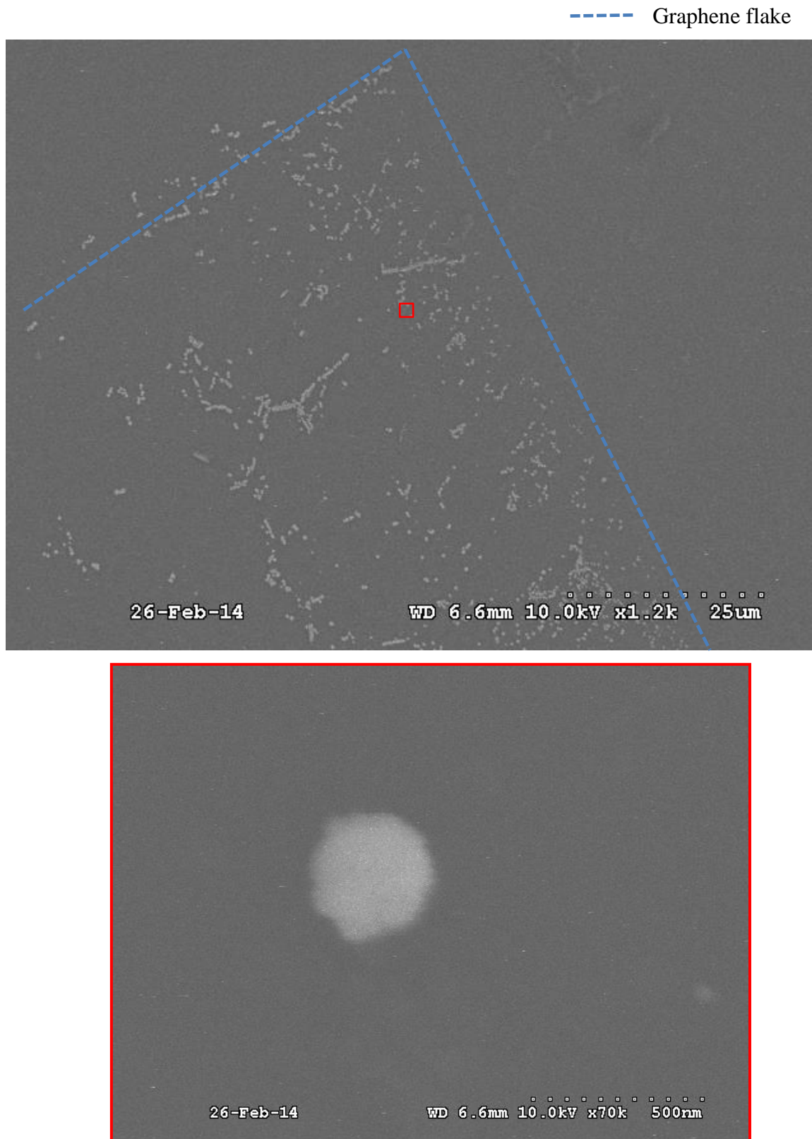
Figure 4.6. Scanning electron microscopy (SEM) pictures of Pt nanoparticles electrochemically deposited on CVD graphene. The red box is a zoom of a nanoparticle structure. This figure is not intended as an in depth characterisation of the nanoparticles, it rather provide an idea of the typical size and distribution of the nanoparticle structures.
