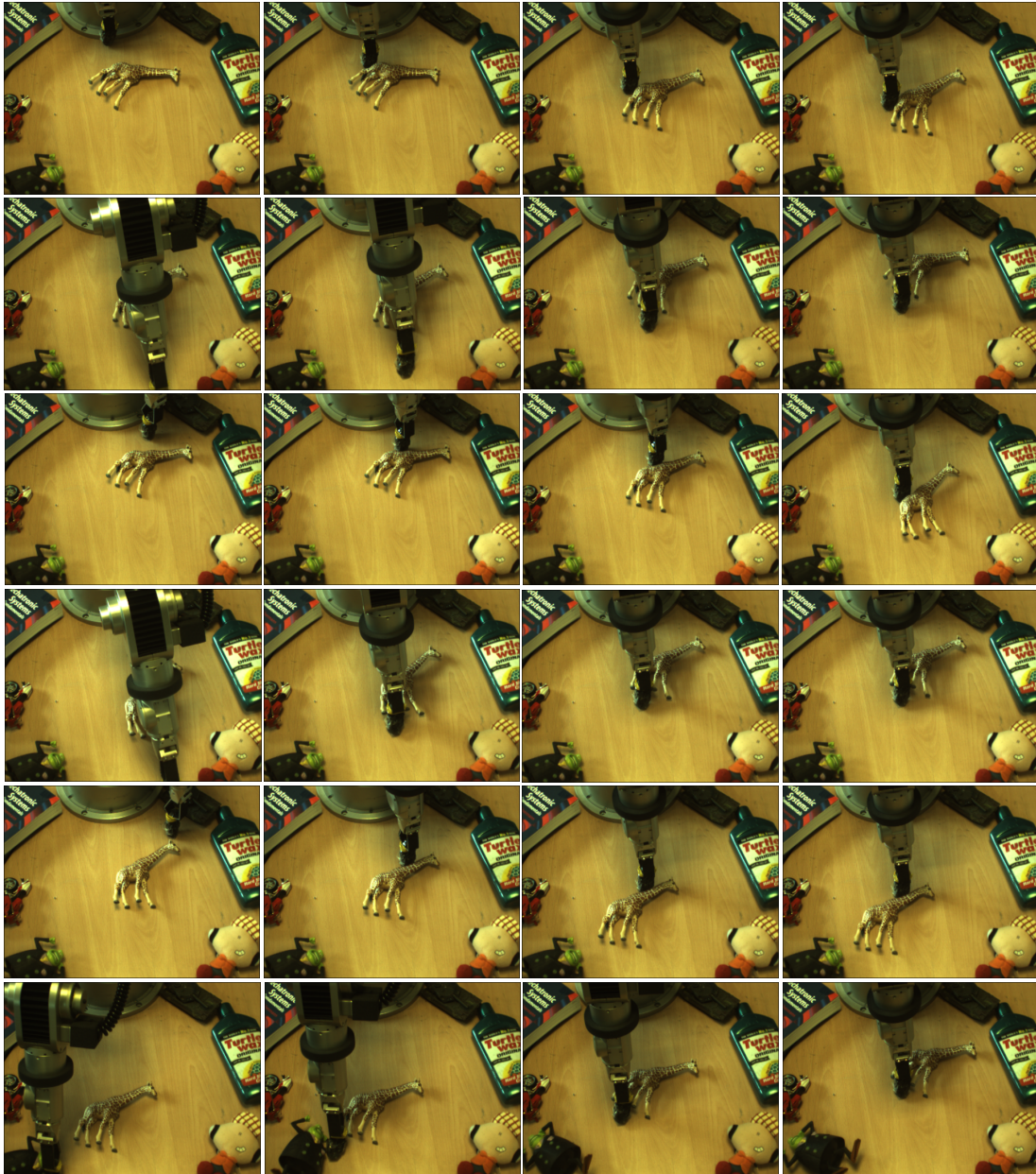
Figure 8-2: Sample frames of the robot manipulating the giraffe object. Each row represents a different push action. The robot continues with this strategy for 10 movements and 3 trials for each object. Note the background clutter and occlusion of the giraffe by the robot arm in several frames of the sequence.
