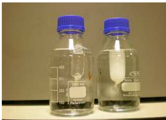
Figure 7.6 RG504/DMSO mixture within the dialysis tubes, dialysed against water. Left bottle: mixture at the beginning of dialysis ( t=0 min). Right bottle: mixture after \sim 2 days of dialysis showing the emulsion formed
