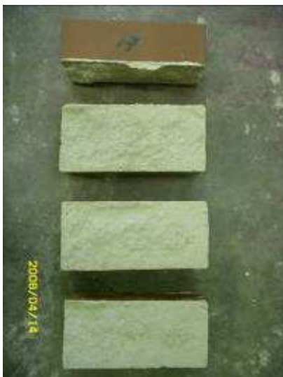
(b) Example of mortar joint failure ('Cheddar Red (Cattybrook)' brick)
