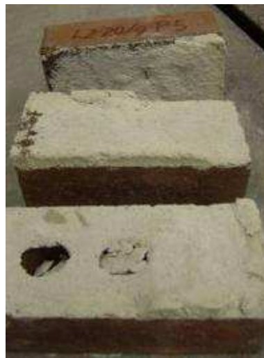
(c) Combined failure
