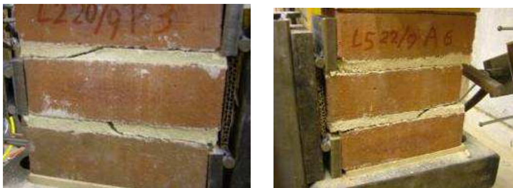
Figure 7.2 Crack patterns in shear test mortar joints
