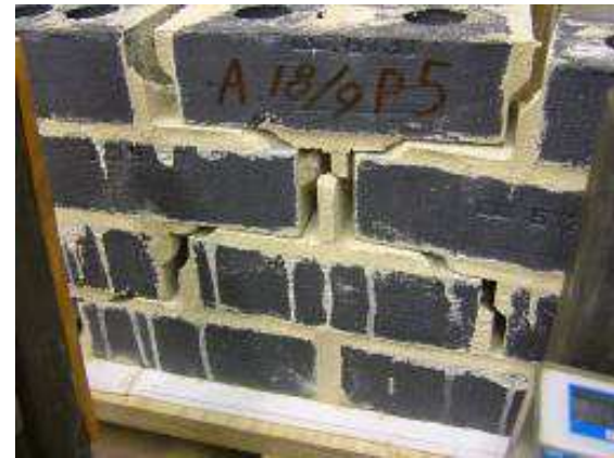
(c) Combined diagonal failure planes
