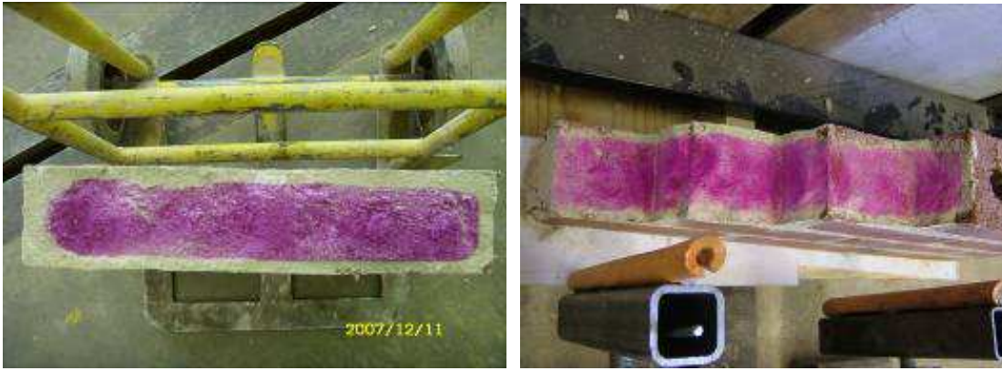
Figure 5.9 Carbonation indicator patterns in 'Berkeley Red Multi' brickwork mortar joints
