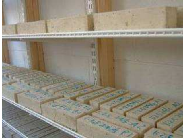
Figure 3.10 Mortar specimens on shelves curing in climate room
