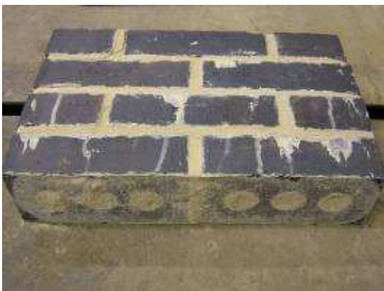
Figure 5.3 Failure modes using low (left: 'Staffordshire Slate Blue Smooth') and high (right: 'Hardwicke Welbeck Autumn Antique') absorption bricks
