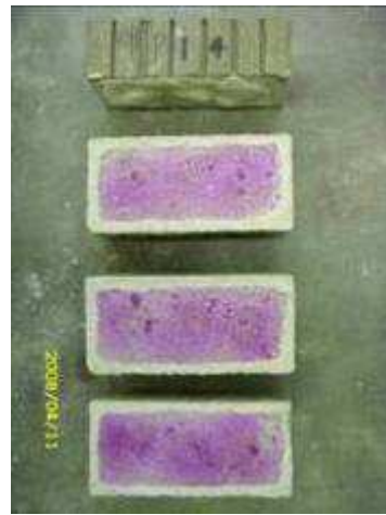
(b) Brunswick Tryfan Grey (Cattybrook) 24-h total water absorption: 3.9% IRA: 0.9 kg/m 2 /min
