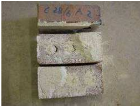
(a) Interface failure
