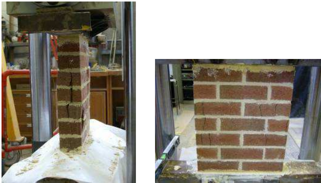
Figure 7.17 Failure mode of masonry in compression
