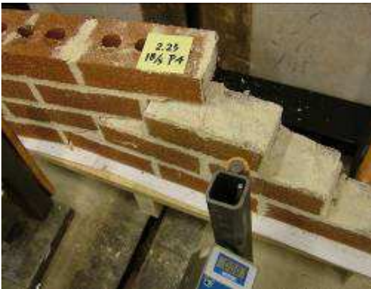
(c) Combined diagonal failure planes
