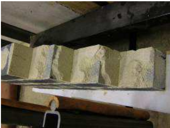
(b) Interface failure in low absorption 'Staffordshire Slate Blue Smooth' walls
