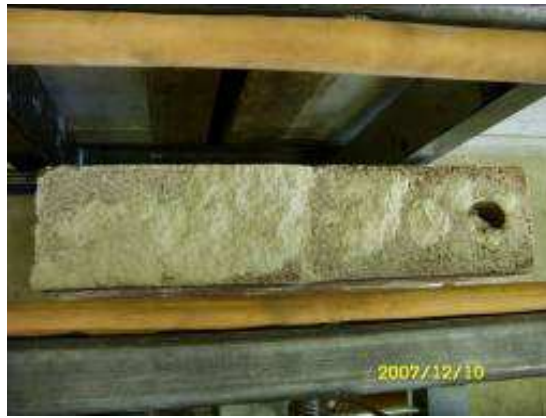
(b) Combined interface and mortar failure
