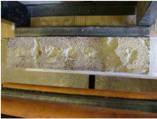
(a) Interface failure
