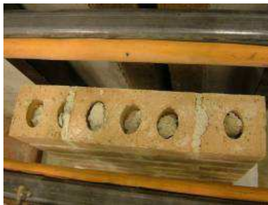
Figure 5.3 Failure modes using low (left: 'Staffordshire Slate Blue Smooth') and high (right: 'Hardwicke Welbeck Autumn Antique') absorption bricks
