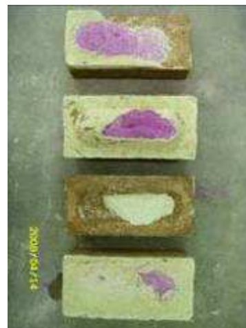
(f) Dorset Red Stock (Ellistown) 24-h total water absorption: 12.7% IRA: 2.1 kg/m 2 /min
