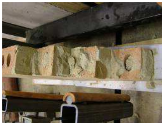
(c) Interface failure for high absorption 'Hardwicke Welbeck Autumn Antique' walls
