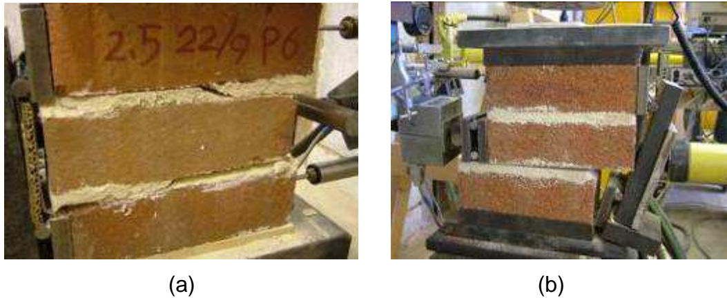
Figure 7.1 Shear test specimens after failure
