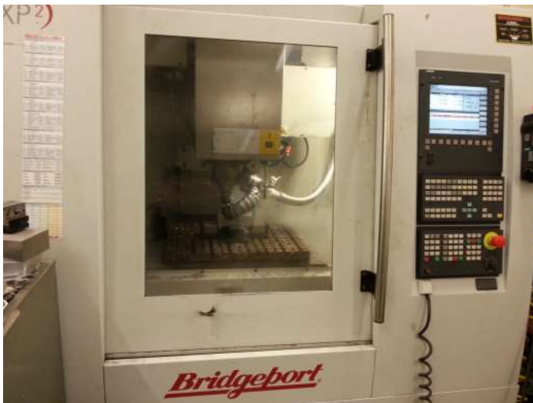
Figure 5.3 The Three-axis CNC vertical milling centre (Bridgeport VMC 610XP 2 ) with cryogenic nozzle system installed and ready for conducting machining experiments.
