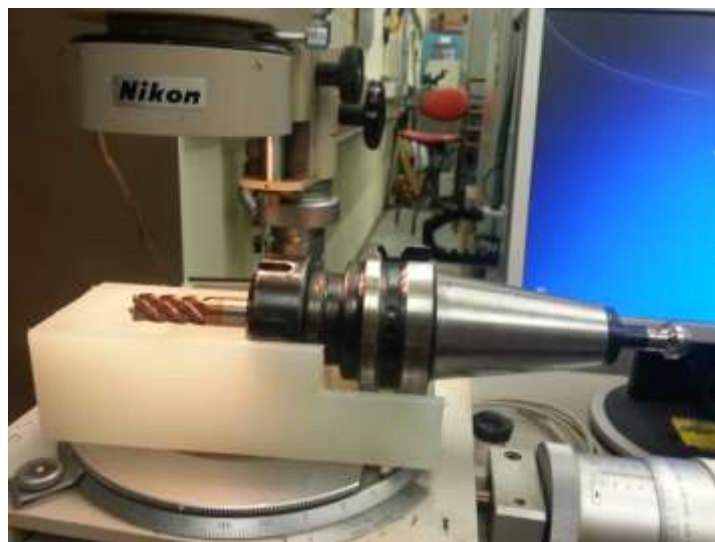
Figure 5.10 Cutting tool with its BT-40 holder carried by plastic holder on the stage of microscope for measurement of tool wear.
