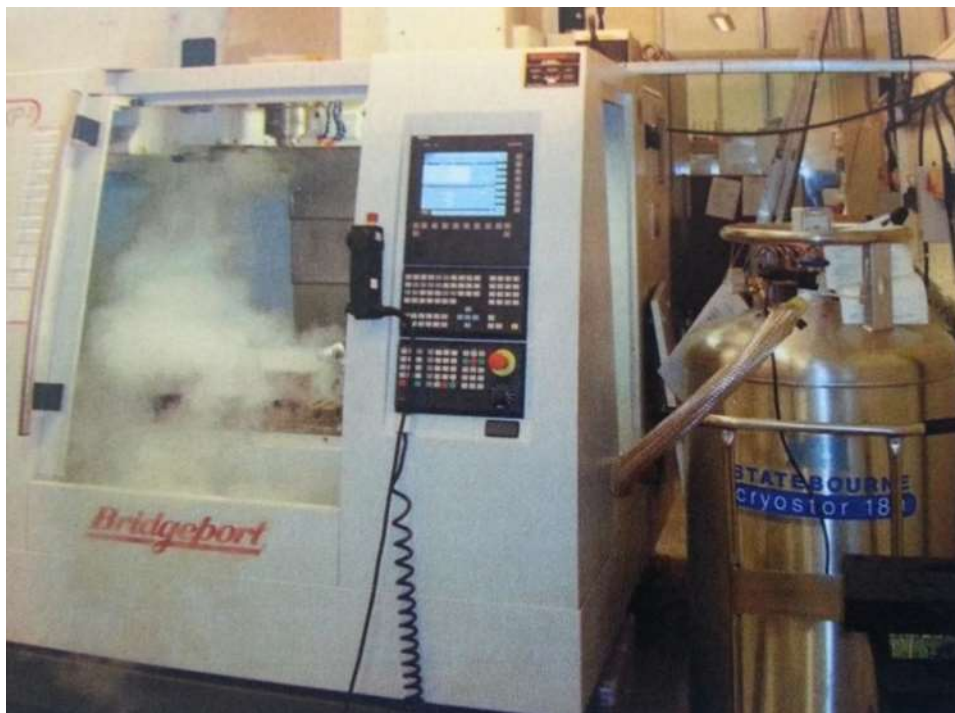
Figure 3.2 Photographic illustration of cryogenic delivery system used in this research (Dhokia 2009; Shokrani 2014)
