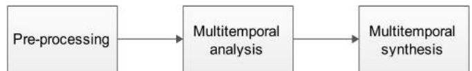
Fig. 2: Multitemporal synthesis general workflow. Pre-processing is necessary to obtain images spatially and radiometrically comparable, thus suitable for the fusion. Analysis is devoted to the extraction of the temporal features involved into the synthesis.
