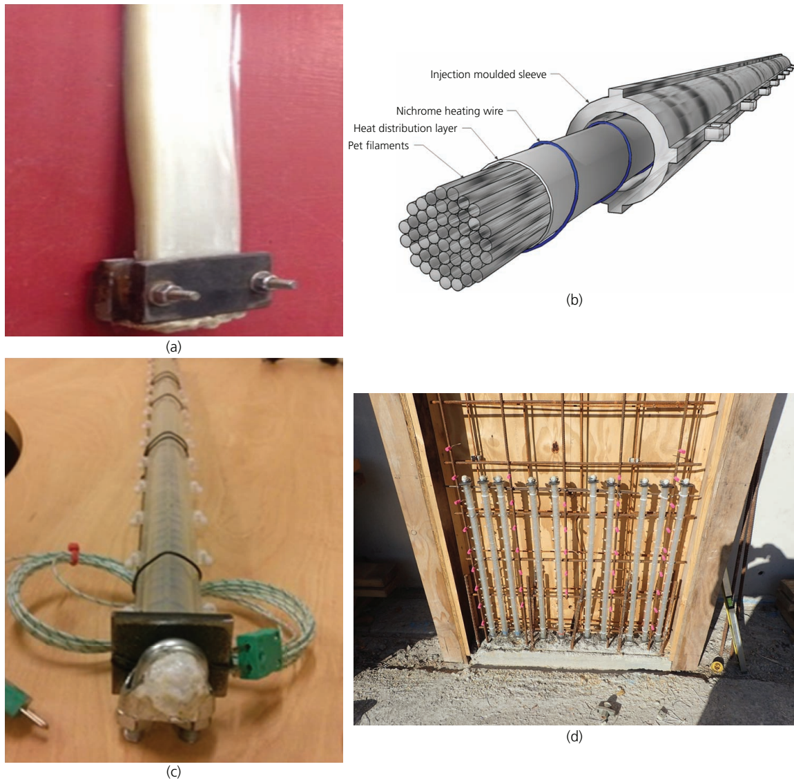
Figure 4. SMPs for self-healing: (a) a typical example of an SMP shape (Teall, 2017); (b) SMP (Davies et al. , 2018) and (c) tendon assembly developed and tested within cementitious matrices; (d) a section of a wall showing the installed SMP and vascular networks (Davies et al. , 2018)
