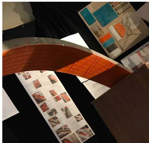
Figure 9. Orange fiberglass formwork creating the patterned underside of the arch.
