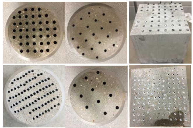
Figure 2. HSCRPC samples (cylinder samples left and cube samples right) containing different amount of vertical pore channels.
