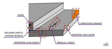
**Figure 1** Illustration of typical material defects monitored by IRT for composite aircraft and spacecraft structures (a), jet engine turbine blades (b), honeycomb panels (c) and metallic aircraft and spacecraft components (d).
