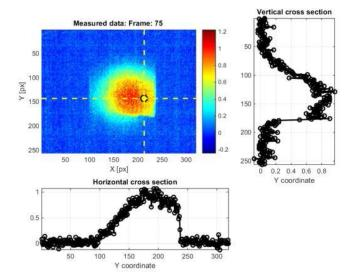
Figure 10 Laser-spot thermography result on fatigue damaged aluminium sample, from [96].
