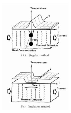
Figure 20 Illustration of the "singular method" (a) and the "insulation method" (b), from [31].
