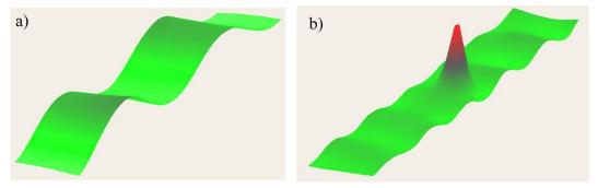
Figure 15 Vibration patterns at the GFRP specimen at 3.4 kHz (a) and at the LDR frequency, 20.9 kHz, on a GFRP sample (b), with permission from [122].
