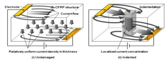
Figure 21 Schematic of the technique developed by Suzuki et al: difference in the path of the electrical current in the case of undamaged and indented areas, with permission from [154].
