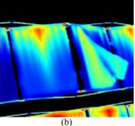
Figure 3 PT results obtained during EVA inspections of a CFRP component of the Space Shuttle (a) and a damaged ISS radiator (b), from [63].
