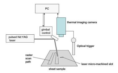
Figure 9 Experimental set-up for laser scanning thermography, with permission from [90].
