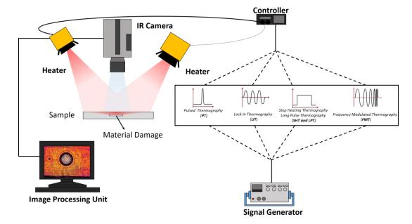
Figure 2 Schematic diagram of optically stimulated thermography (OST).
