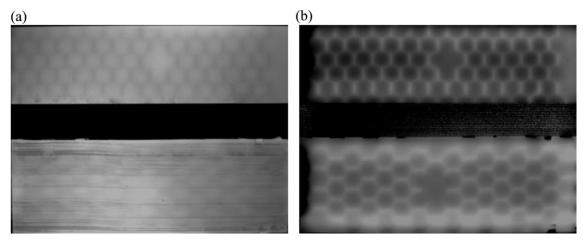
Figure 7 Lock-in thermography testing of a titanium alloy honeycomb sandwich structure with disbond, with permission from [75].
