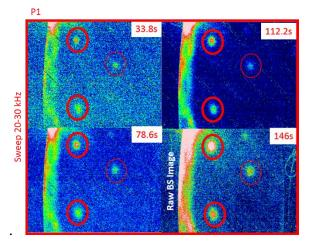
**Figure 16**. Nonlinear ultrasonic stimulated results thermography on a composite stiffened panel while conducting a sweep between 20 kHz and 30 kHz, with permission from [28].
