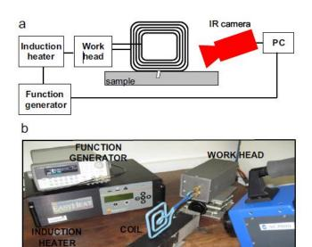
Figure 17 Experimental set-up of pulsed eddy current stimulated thermography, with permission from [131].
