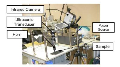
Figure 11 Experimental set-up of ultrasonic stimulated thermography, from [101].
