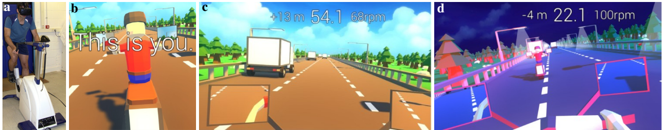
Figure 1: a) The exergame is based on a computer-controlled stationary exercycle and played while wearing a head-mounted display. b) A “self modelling cue” helps the player to identify a “ghost” avatar with their own previous performance. c) Low-intensity cycling and avoiding trucks during warm-up, recovery and cool-down phases. d) High-intensity race against the “ghost.”
