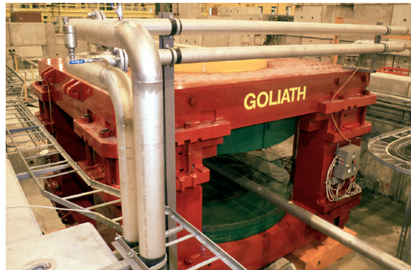
Figure 4.7: Photograph of the Goliath magnet in the H4 experimental area at CERN.
