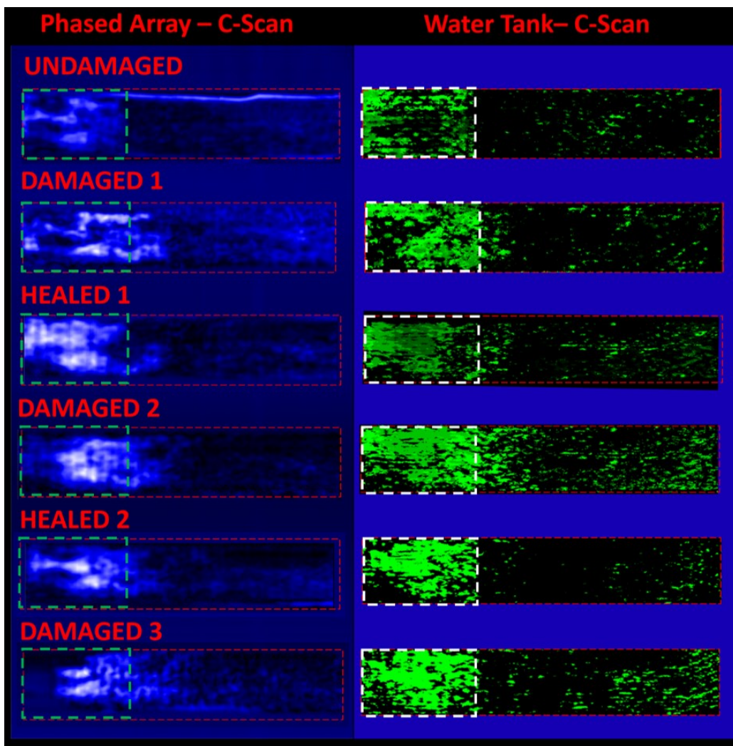
17 Figure 16: Phased array (5MHz) vs. Water Tank C-Scan (35MHz) S1
