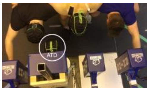
Fig 1: Experimental setup including an ATD positioned between scrum machine beams in the hooker position.
