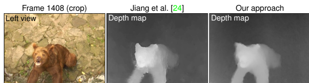
Figure 9. Comparison of depth maps for the BEAR sequence by Jiang et al. [24] and our approach. Our variational refinement produces smoother depth variations on the bear and the background, and only slightly blurrier depth boundaries.
