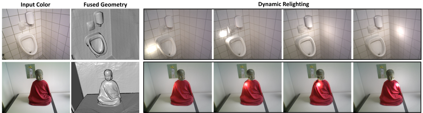
Fig. 11. Dynamic geometry-based relighting. A virtual shading image is generated by rendering the scene geometry under a new light source. The resulting shading map is blended with the shading layer before recombining it with the reflectance to obtain a relighting effect.
