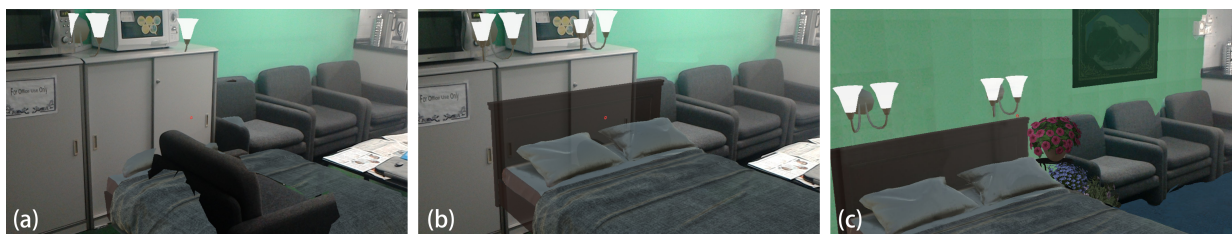
Figure 16. Comparison between different MR experiences. (a) Virtual models (the bed) can collide with the real objects (the sofa) in the current mixed reality solution in Hololens. (b) Overlay virtual models on top of real scene results in ambiguous spatial relation. The bed is actually aligned to the wall as the cabinet, but it looks like in front of the cabinet. (c) Enhanced mixed reality experience enabled by SceneCtrl . Cabinet and sofa are deleted from the scene. (Images are captured using the RGB camera feed from Hololens.)
