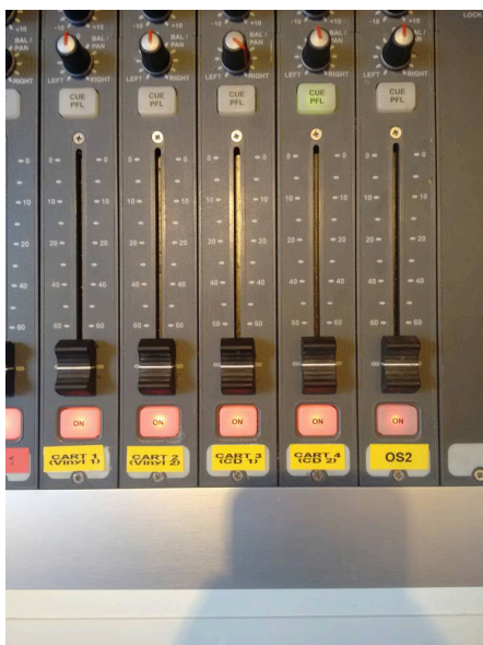
Fig. 5.5 URB - Studio Mixing Desk
