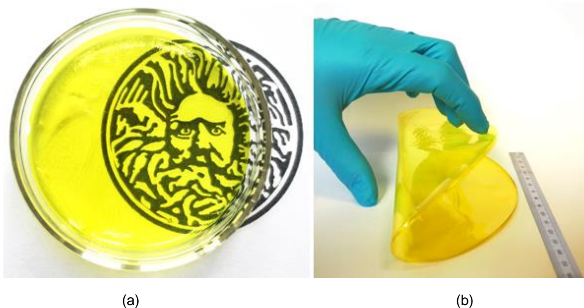
Fig. 1 Bright yellow transparent PIM-1 film cast in a Petri dish over University of Bath logo shortly after evaporation (a), PIM-1 film after removing from Petri dish (b).
