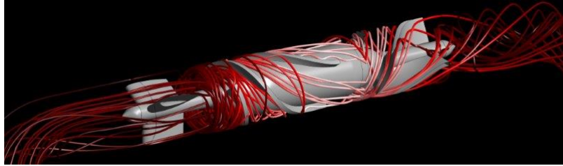
Figure 5: Pathlines through the HeartMate II VAD
