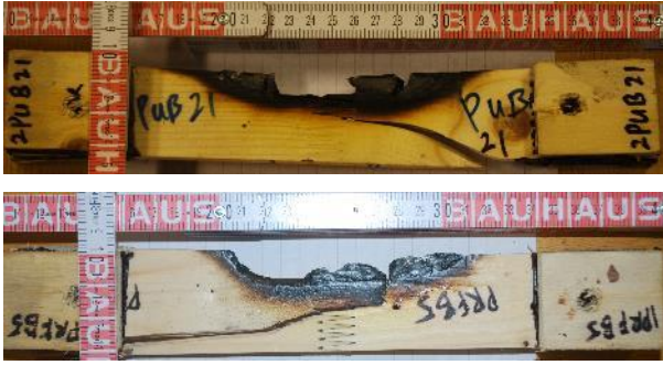
Figure 13: Failures near knots (top) and along the slope of grain (bottom)
