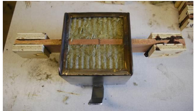
Figure 6: Stone wool protecting the sides of the specimen
