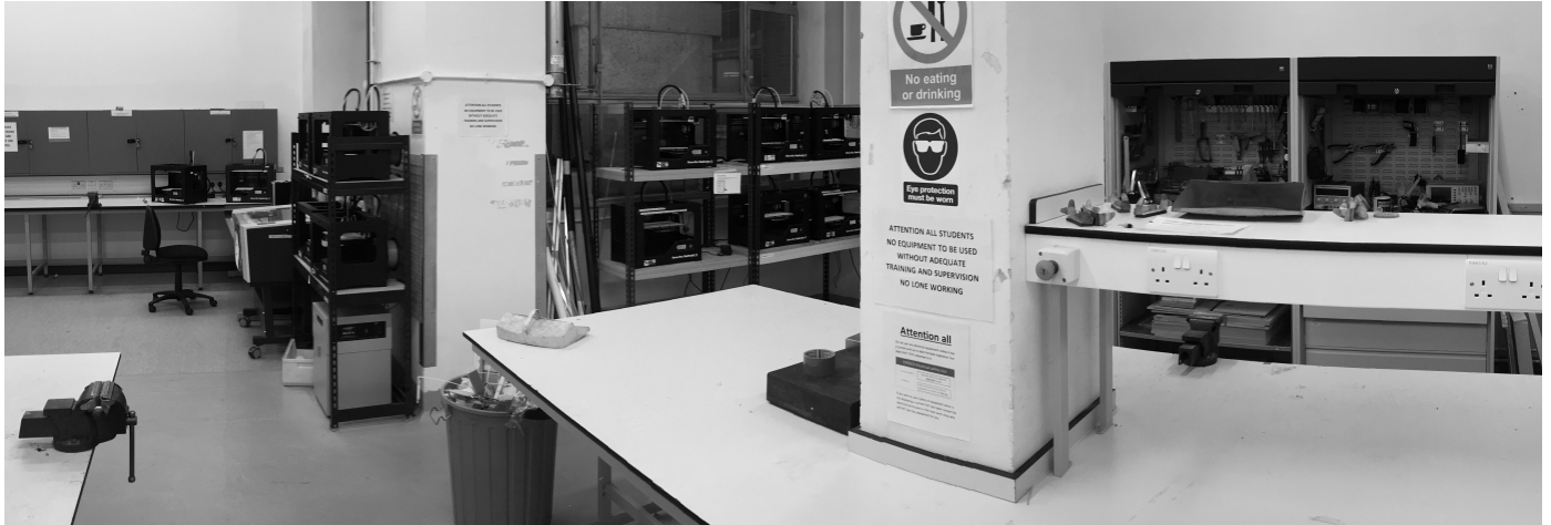
Figure 1: The FabLab at the University of Bristol featuring lathes, pillar drills, fixtures store, laser cutters, 3D printers, workstations and hand-tools store.
