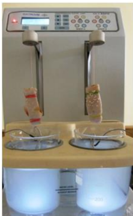
Figure 5. Workflow presents the mucoadhesion study of drug loaded single and dual crosslinked pectin-alginate beads using USP tablet disintegration test apparatus in Tyrode's solution at 37 \pm 0.5^\circ\text{C} .
