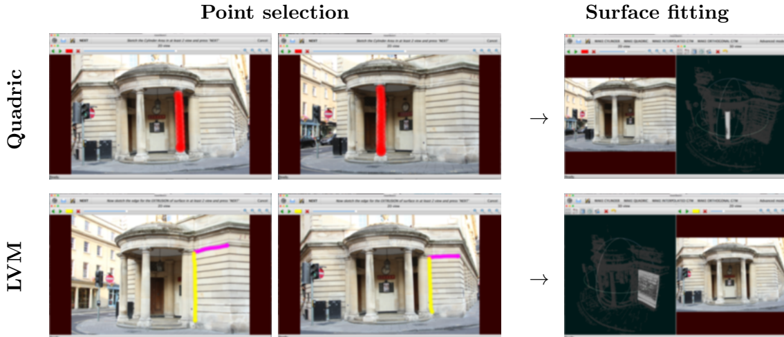
Figure 2: An example of some sketch input to the system and the corresponding output from the primitive fitting algorithms. The first row contains an example of fitting an ellipsoid to a column of a building, and the second row is an example of a perpendicular extrusion using a pair of latent variable models.
