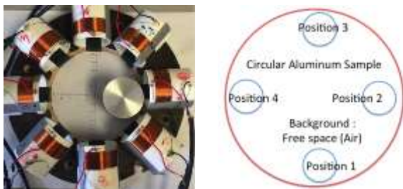
(a) Real conductive distribution in position 1 (b) Circular aluminum sample in position 1,2,3,4 Figure 9. Experimental setup.
