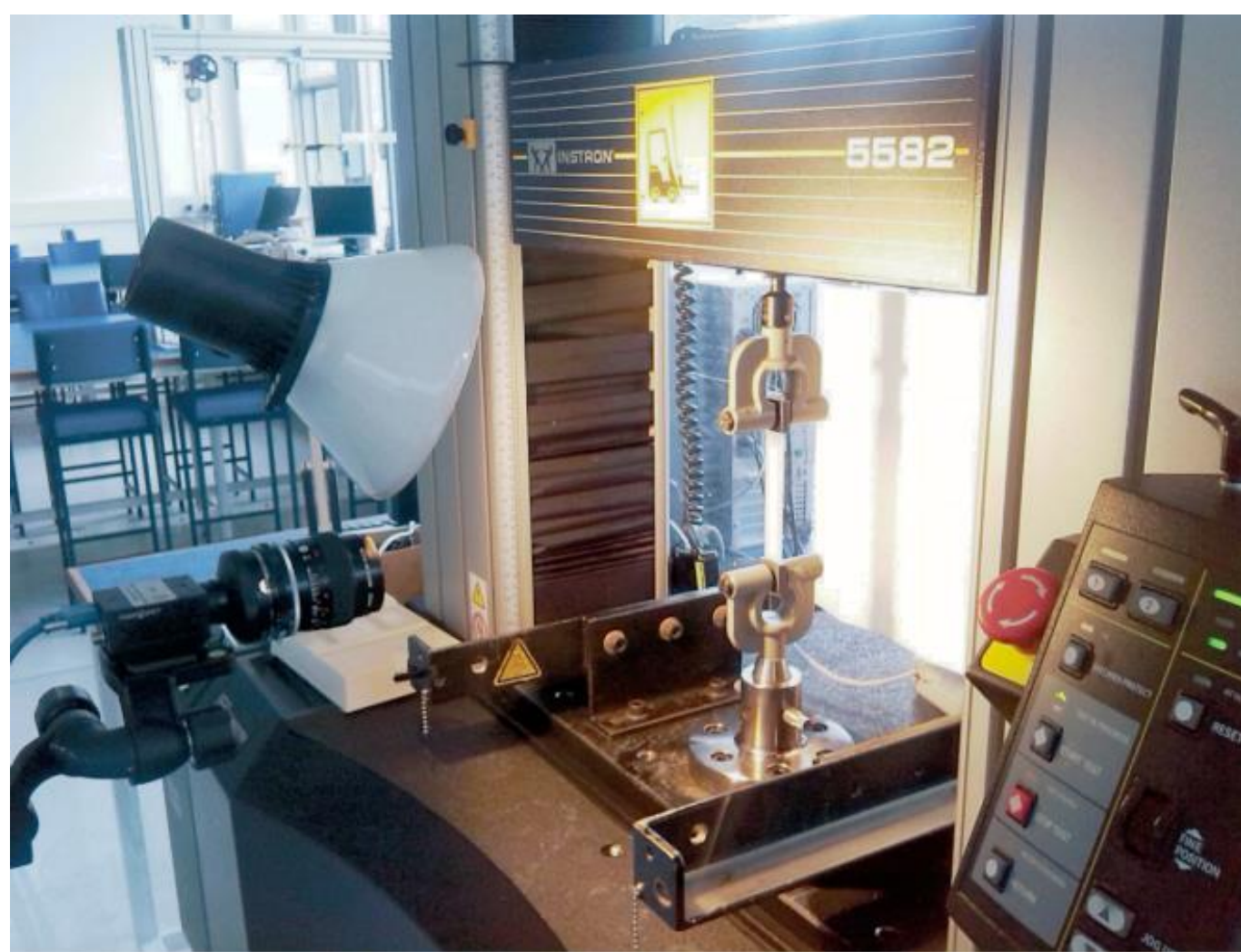
Fig 2: Viscoelastic characterisation of the UHMWPE
