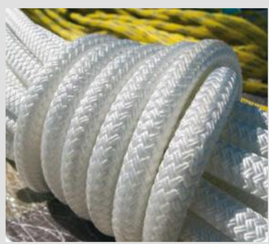
Fig 2. Braided construct of UHMWPE fibre [3]
