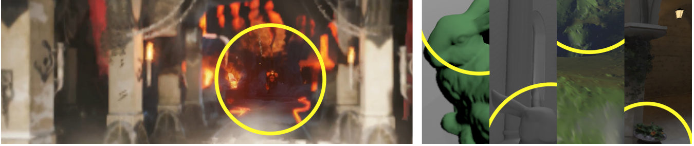
Figure 1: Left: Our foveated resolution method running on a commercial video game engine. Right: Our foveated resolution, ambient occlusion, tessellation, and ray-casting (respectively) methods. Areas outwith the circles are the peripheral regions rendered in lower detail.
