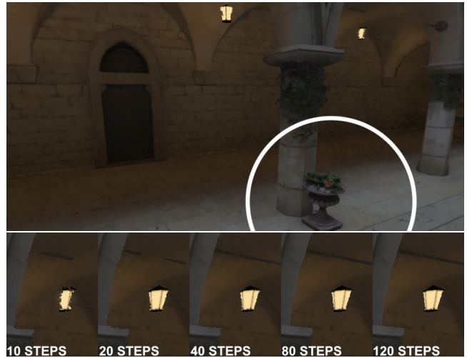
Figure 5: Top: Sample frame from our ray-casting method with 120 per-pixel steps in the foveal region (within circle) and 10 per-pixel steps in the peripheral region (outwith circle). Bottom: Close-up of right lamp showing artefacts across different quality levels.
