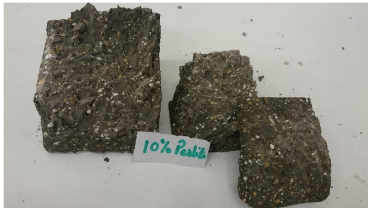
Figure 3 Broken cube showing good distribution of perlite (the white spots) in concrete M2
