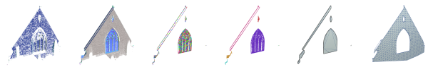
Figure 3: Intermediary data exploited by the ARROW algorithm to produce the result displayed in figure 1 - illustrating (from left to right, top to base) quantized wall-point filter response, binary division resulting from the SDF-split (wall-points in gray, deviant-points in blue), KD-tree used to 'chunk' sets of deviant points, connected component clusters extracted from KD-tree chunks, railed surface-element models, and finally quad-dominant wall model.
