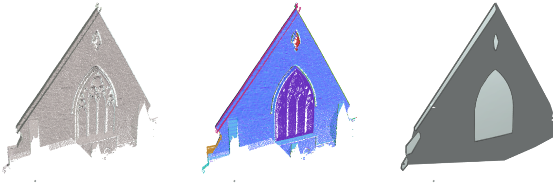
Figure 1: ARROW → Accurate Railed Reconstruction of Openings and Walls : (left) input unstructured points, (middle) signed-distance-field-split with segmented elements, (right) the output polygon-mesh (composed of a quad-dominant wall and railed surface-elements).
