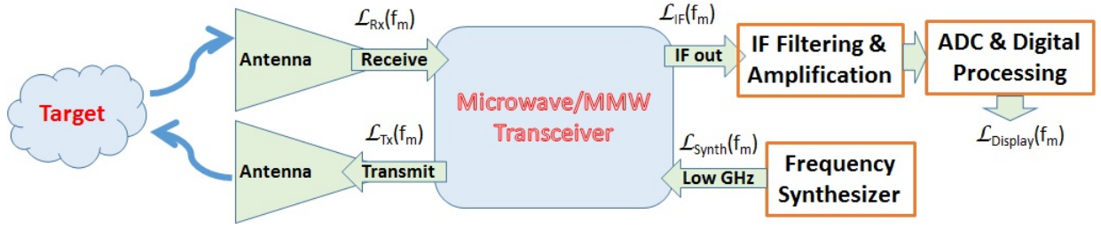
Fig. 1. Block diagram showing phase noise propagation in a radar system.
