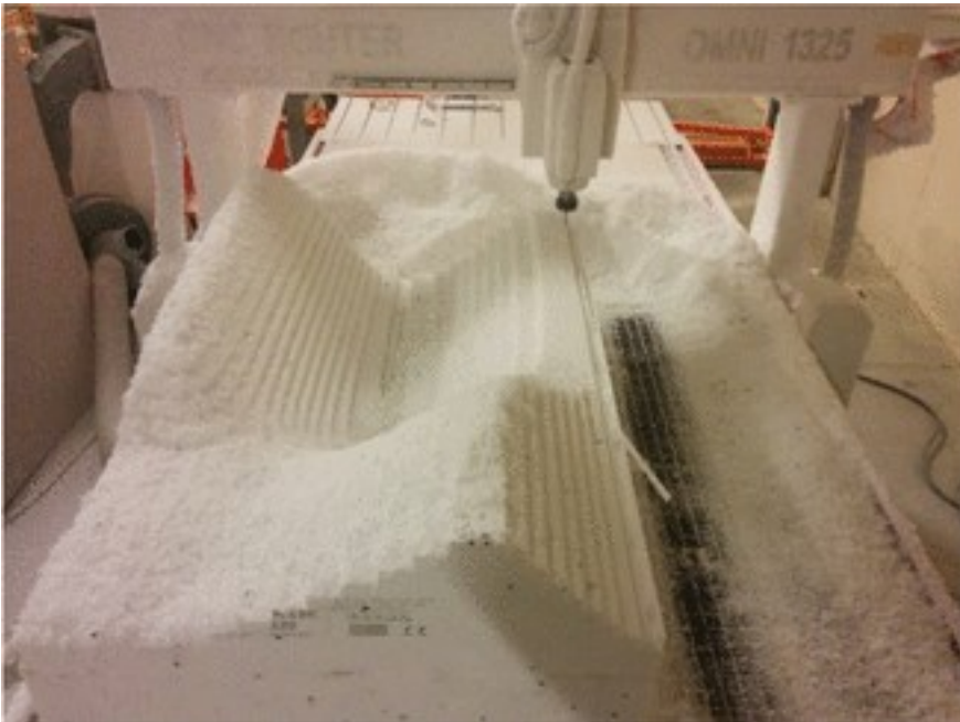
Fig. 8 Concrete mould milled by a CNC machine.
