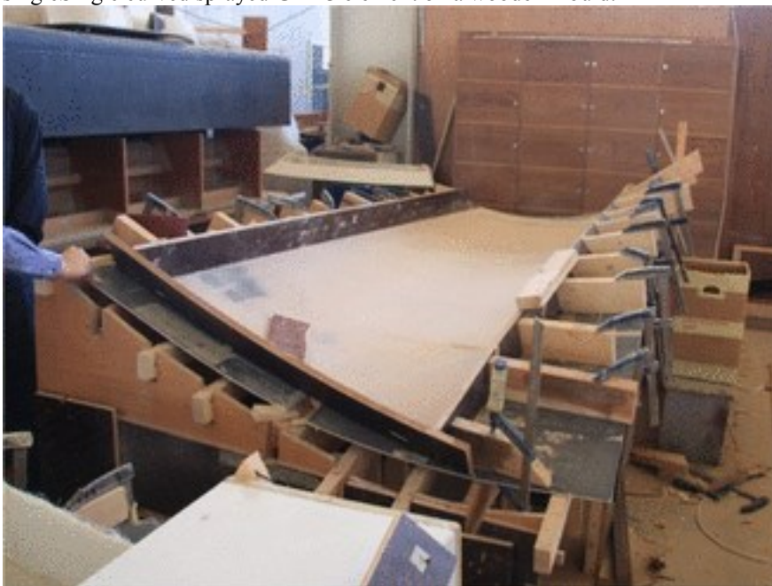
Fig. 1 singleSingle curved sprayed GFRC element on a wooden mould.
