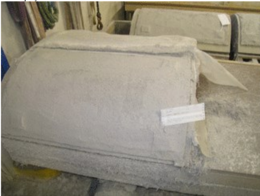
Fig. 1 singleSingle curved sprayed GFRC element on a wooden mould.
