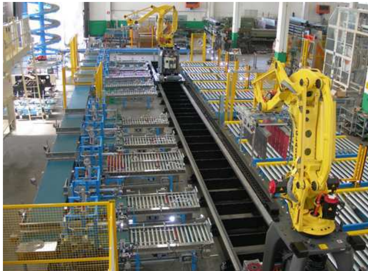
Figure 1. An industrial example of twin robots on a rail (AllGlass 2017).
