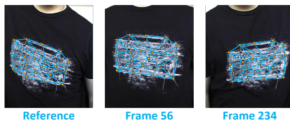
Fig. 1. A mesh is tracked through a long nonrigid sequence by using our method.
