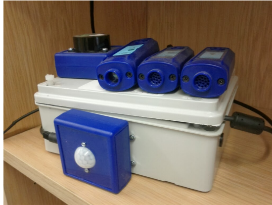
Figure 2: Sensor box in situ , showing PIR, temperature, CO 2 , light, sound and humidity sensors.
