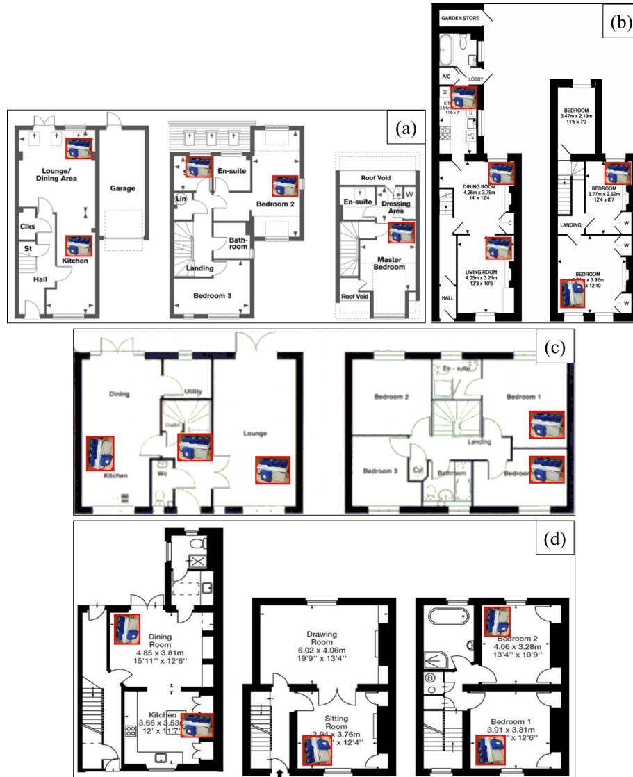
Figure 1: Experimental Settings – The placement of sensors at each home: (a) Home A – 3 Bedrooms, 3 Floors, (b) Home B – 3 Bedrooms, 2 Floors, (c) Home C – 4 Bedrooms, 2 Floors and (d) Home D – 4 Bedrooms, 3 Floors in Table 1
