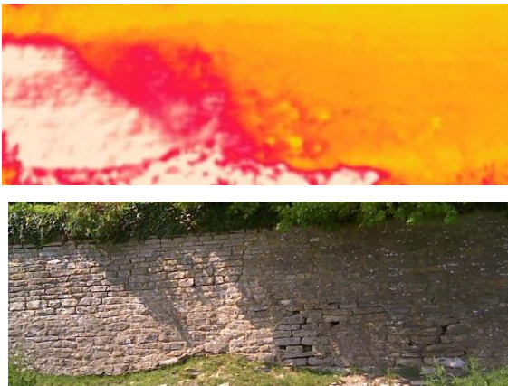
Figure 6: Thermal image showing the effect of shading.
