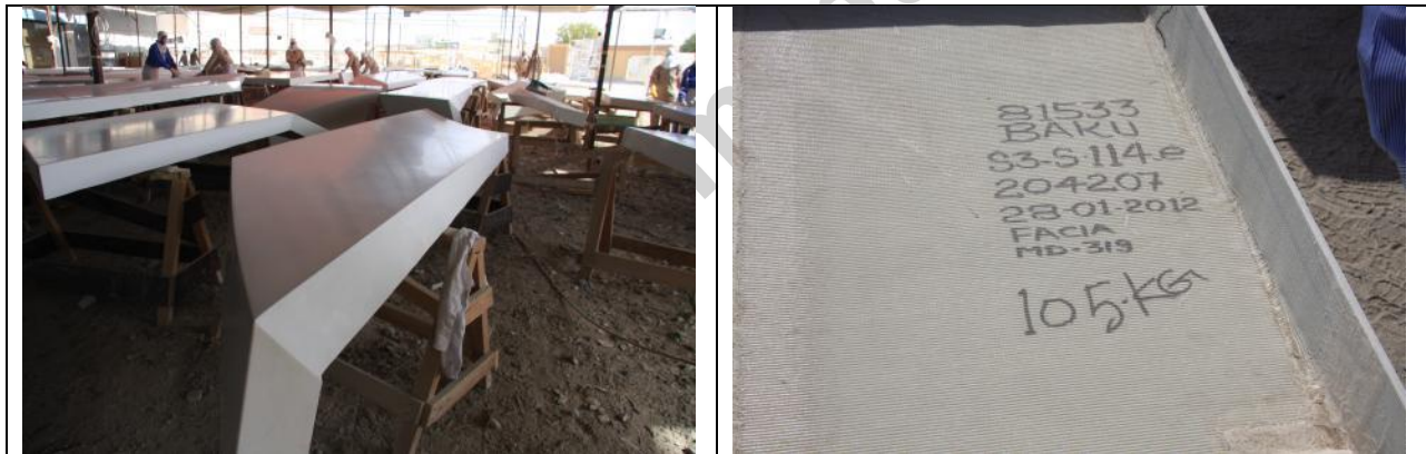
Figure 4 Production of GFRP cladding panels for the Heydar Aliyev Center
