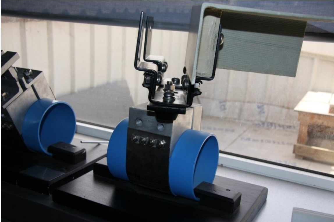
Figure 8 The connection between the secondary steel and the GFRP panels used on the Heydar Aliyev Center, which enables to accommodate tolerances between the secondary substructure and the complex geometry panels.
