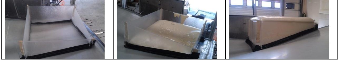
Figure 10 The proposed new approach which adds an additional step between the flexible table and the casting of the GFRc element.
