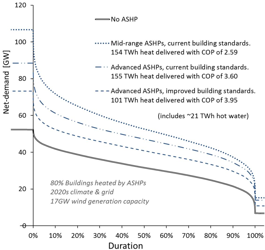
Figure 6: Net-demand duration curves for different operating conditions
