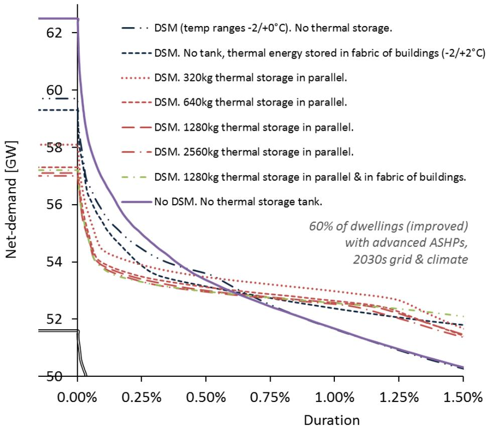
Figure 8: Net-demand duration curves with different thermal storage options
